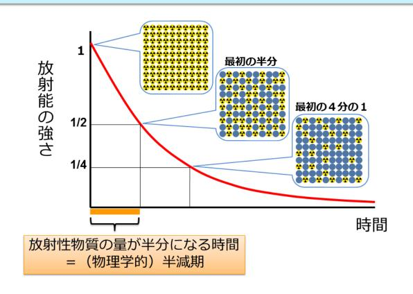
Half Time and decreasing the radiogenic element The ordinate is radiogenic strength (amount of radiogenic element). The abscissas is time.
