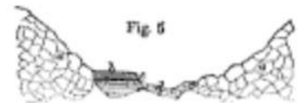
a. Porphyry. b. Coal series. c. Coal seams. a. Porphyry. b. Coal series. c. Coal seams. d. Creek rubble.
